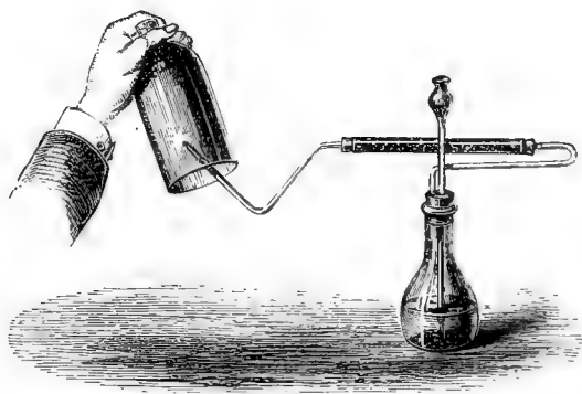
FIG. 29.—Formation of water by combustion of dry hydrogen.
