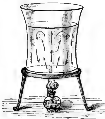
FIG. 46.—Currents in water by heat.
