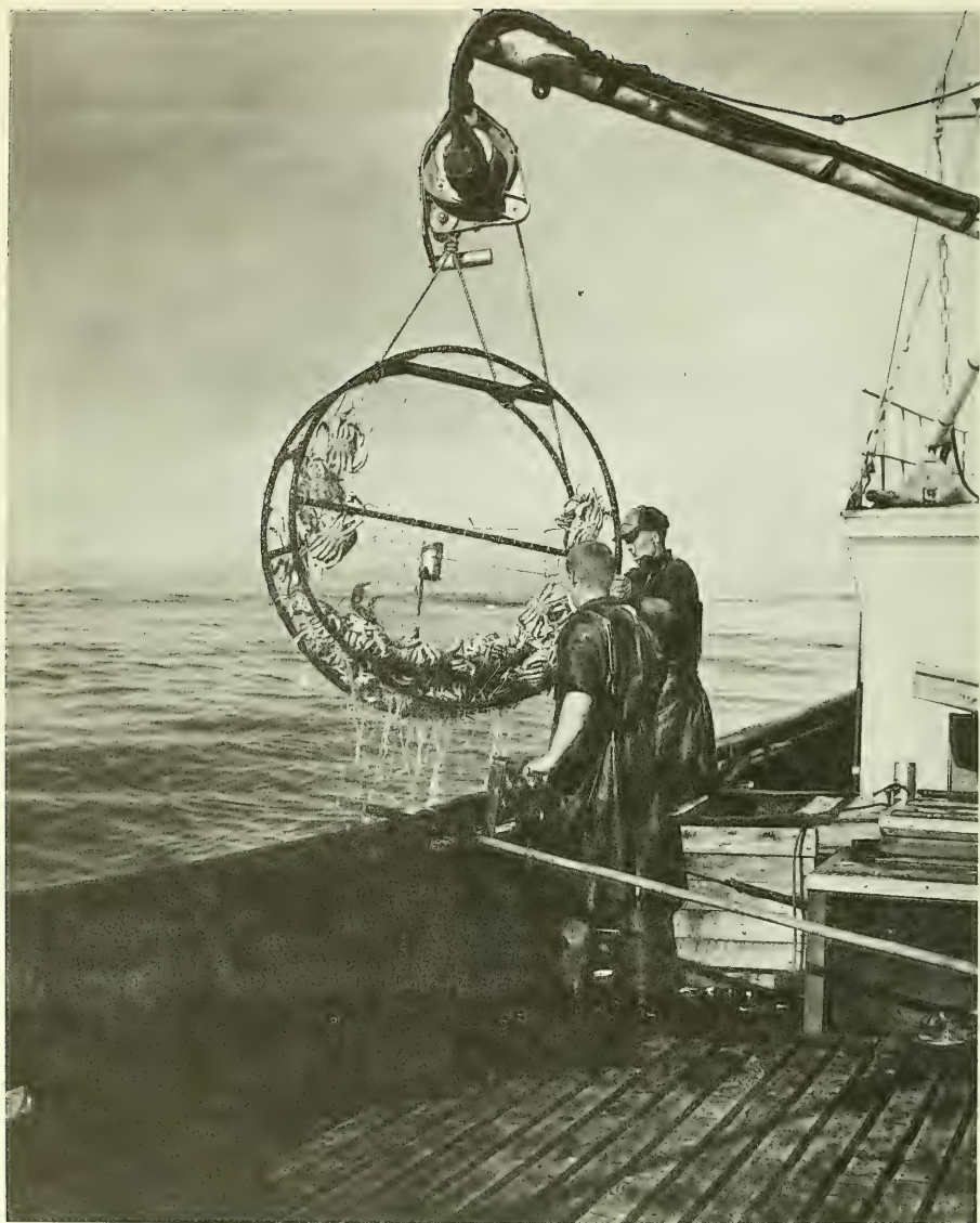
Fishermen guide dungeness crab pot (60-inch diameter) being lowered by boom to power barge. See Article p. 44. (Robert M. Meyer)
