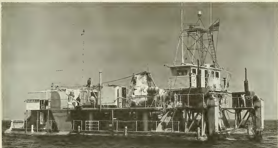
Fig. 3 - Alvin's mothership, Lulu, is a catamaran. Alvin is launched and retrieved from a cable suspended between the hulls. In this picture, Alvin has been raised to working deck.
