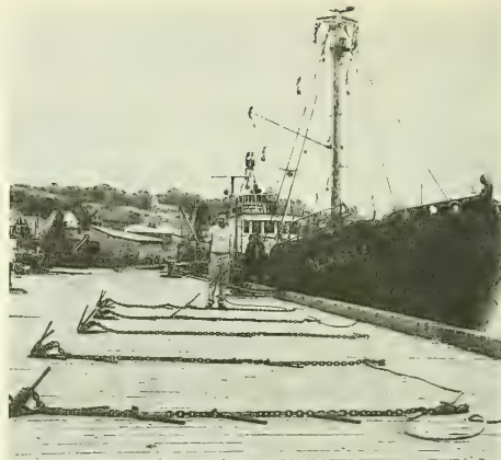
Fig. 1 - The grapnel "array" used to retrieve 19 lobster pots lost in 175 to 210-fathom depths on the Continental Slope.
