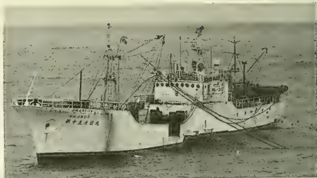
Fig. 3 - A Japanese Danish seiner in eastern Bering Sea. A fleet of 12-15 accompanies a factoryship engaged in production of fish meal, oil, and minced fish meat. In photo, net has been fastened to working gear on foremast and ship is dead in water. (Photo: J. Branson)
