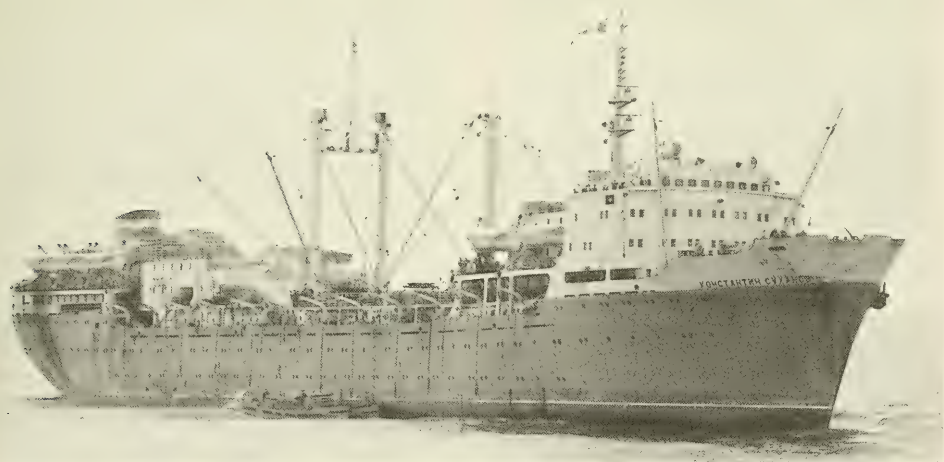
The "Konstantin Sukhanov," a passenger-freighter, was converted to a fish factory ship for crab fishing in the Bering Sea.
