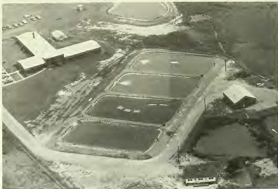
Fig. 1 - Four \frac{1}{4} -acre, man-made, salt-water ponds in front of BCF Biological Laboratory, Oxford, Md. Built above sea level, each pond is about 75 feet by 145 feet by 3.3 feet deep. Each holds about 312,500 gallons of water. The ponds have clay bottoms and sides. Dual pipe and pump systems permit weekly alternations and flushing to prevent fouling.
