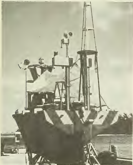
Fig. 1 - Nomad (Navy Oceanographic Meteorological Automatic Device) buoy transmits data up to 2,000 miles over standard 100 words-per-minute radioteletype circuits. (U. S. Navy)
