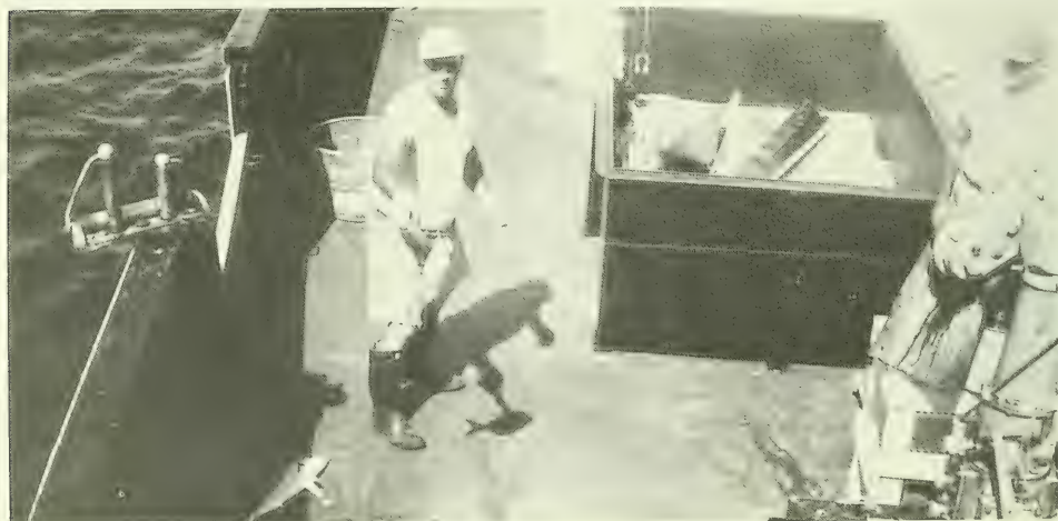
Fig. 3 - Removing small fish from longline. Short gangions went through the roller (on the rail) and longline hauler (right) without fouling.
