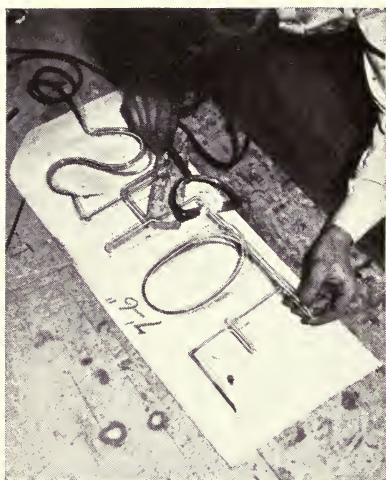
FIG. 53.—Glass blower splicing two letters with hand torch over asbestos layout.
