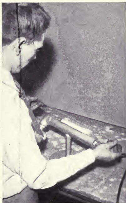
FIG. 43.—Use of ribbon fire. Note method of holding glass as it is rotated in flame.
