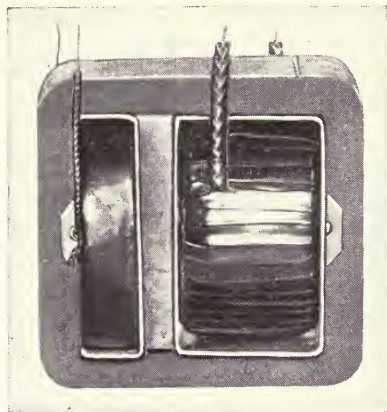
FIG. 21.—Internal construction of low-voltage type (2000 to 5000 volts) neon transformer. Only one magnetic shunt is used, whereas two are usually used in the higher-voltage types (see Fig. 17).
